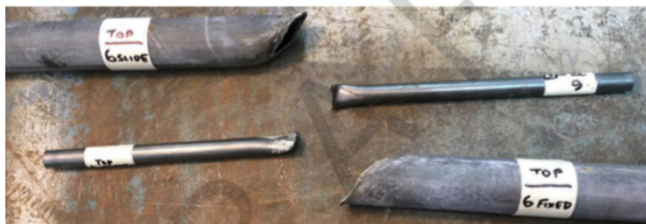
Figure 6.6. Sample 6 – Tubing Completely Parted by Shear Event
