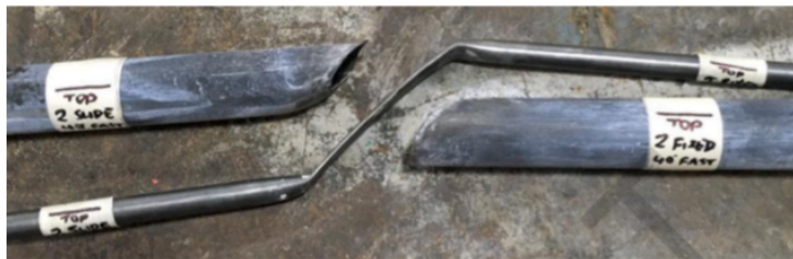
Figure 6.5. Sample 2 – Tubing Deformed by Shear Event
