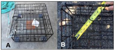
A recreational box-style crab trap (A), with two required 4<sup>1</sup>/<sub>4</sub>-inch escape rings placed on the top of the trap, one with a ring tied in place using No. 120 untreated cotton twine, which serves as the destruct device. When this material corrodes or fails, it will create a large enough opening (B). Photo by J. Langell and J. Hendricks, CDFW.
