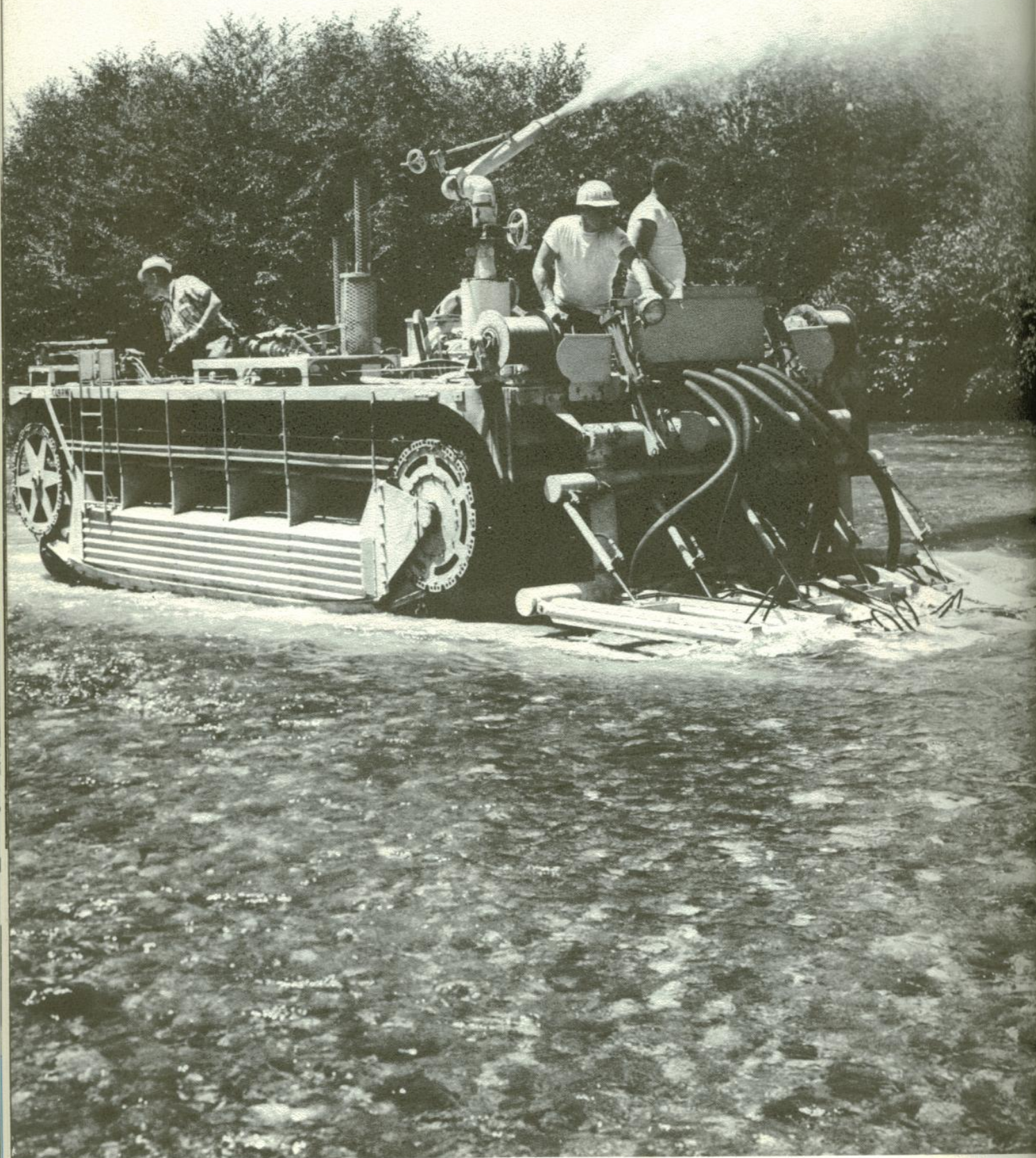
This machine was designed to clean spawning gravel. It works well under some conditions, but cannot cope with the tons of sediment washed into streams by poor land use practices.
